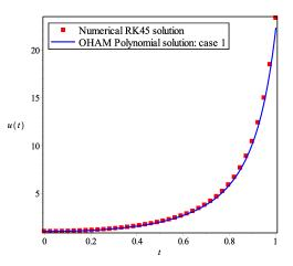
Figure 1: Comparison between the results obtained by means OHAM, Eq. (28) and numerical results: numerical results in solidbox mark and approximate solution in continuun line.
