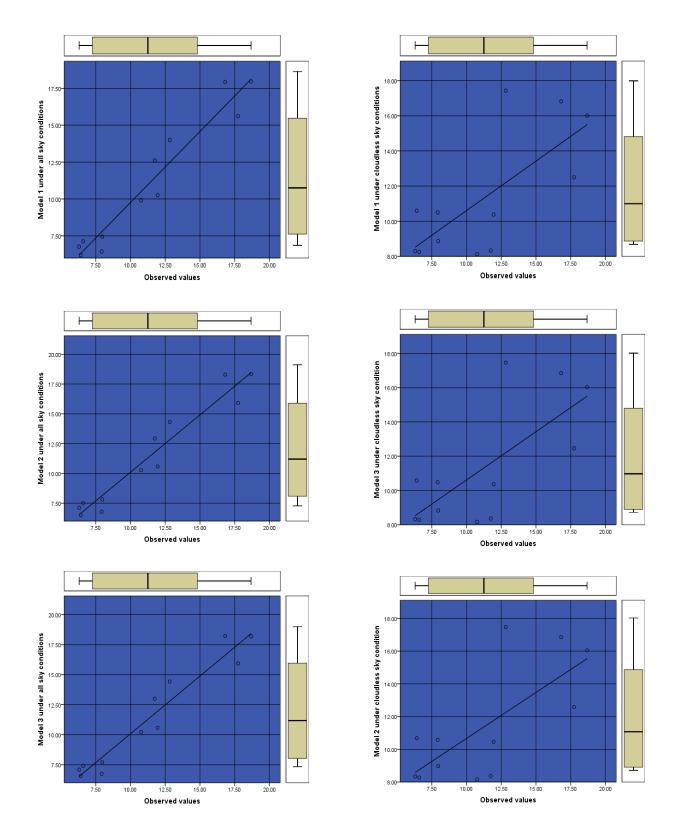
Fig. 6: Scatter Plots and Box diagrams between observed and predicted (models) direct normal irradiance under all sky condition (model 1, 2, 3) and under cloudless sky condition (model 1, 2, 3) for Port Harcourt
