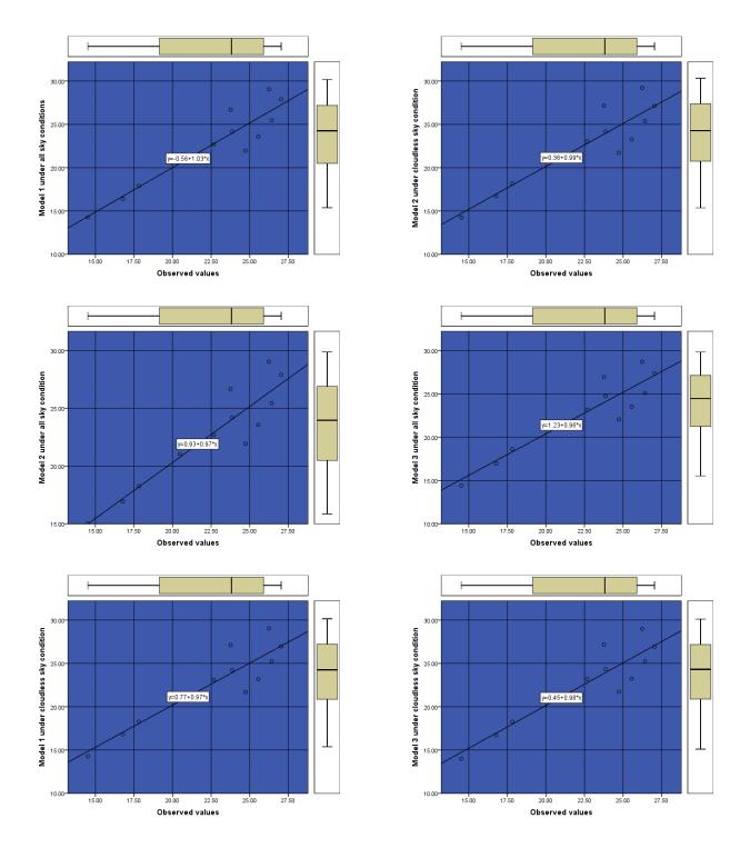
Fig. 10: Scatter Plots and Box diagrams between observed and predicted (models) direct normal irradiance under all sky condition (model 1, 2, 3) and under cloudless sky condition (model 1, 2, 3) for Maiduguri
