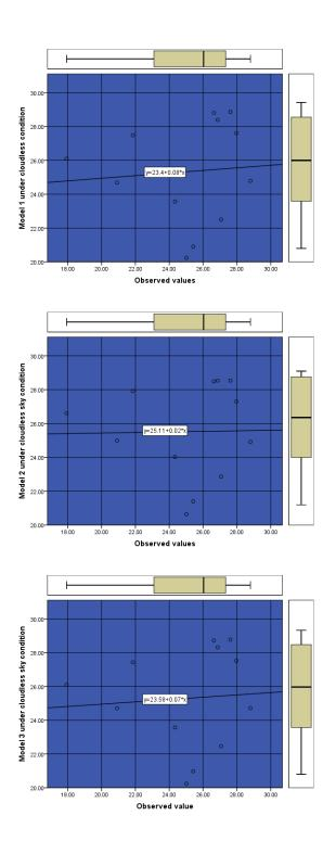
Fig. 11: Scatter Plots and Box diagrams between observed and predicted (models) direct normal irradiance under all sky condition (model 1, 2, 3) and under cloudless sky condition (model 1, 2, 3) for Sokoto.
