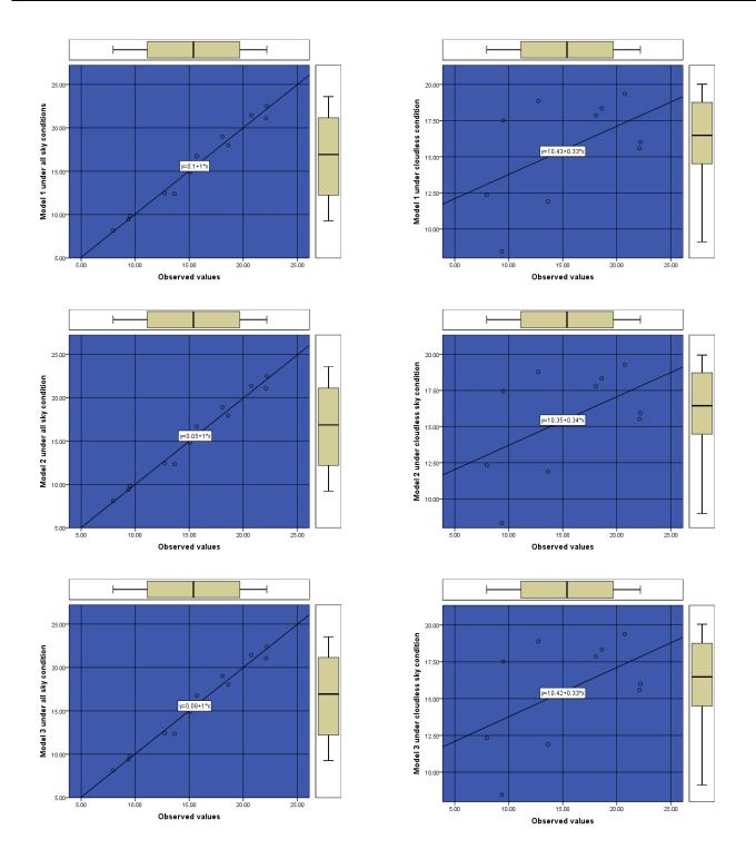
Fig. 8: Scatter Plots and Box diagrams between observed and predicted (models) direct normal irradiance under all sky condition (model 1, 2, 3) and under cloudless sky condition (model 1, 2, 3) for Ibadan
