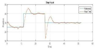
Fig. 11: Real Time Response Proportional- Derivative Integral (PID) Controller.
