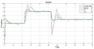
Fig. 14: Comparison between SMC and PID with the Step Signal.
