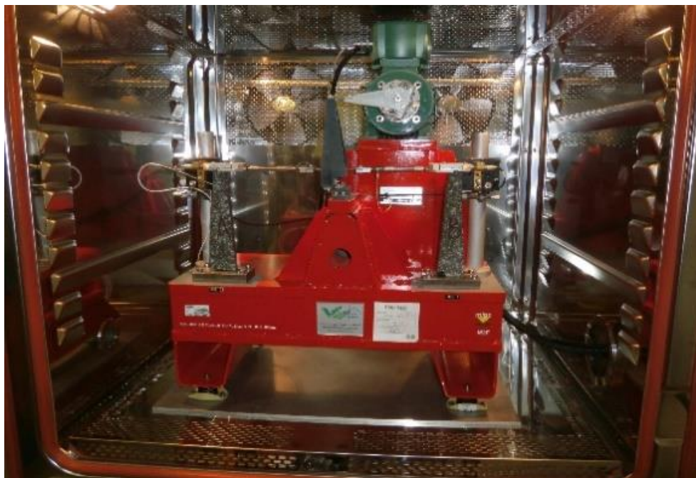
Figure 8: Execution of the fatigue test on 20-EME
