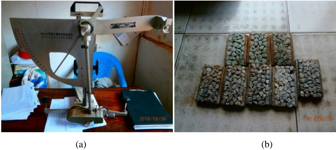
Figure 7: Measurement of the residual roughness after polishing (a), gravel mosaic 6.3 / 10 mm (b)
