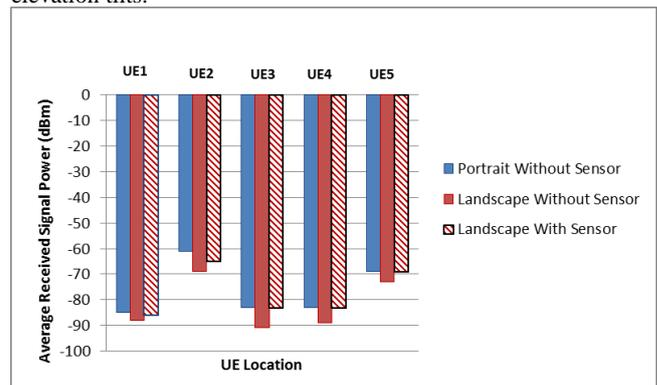
Fig. 7: UE's Average Received Signal Power at various locations.
