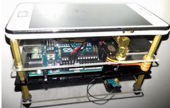
Fig. 5: The handset with integrated sensor.
