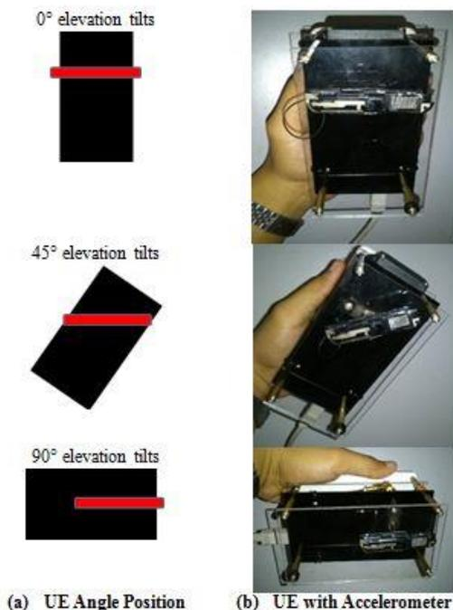
Fig. 6: UE elevation tilts.
