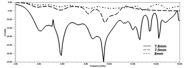
Fig 8: Return loss by varying length of feed
