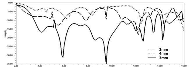
Fig 9: Simulated Return loss by varying feed width
