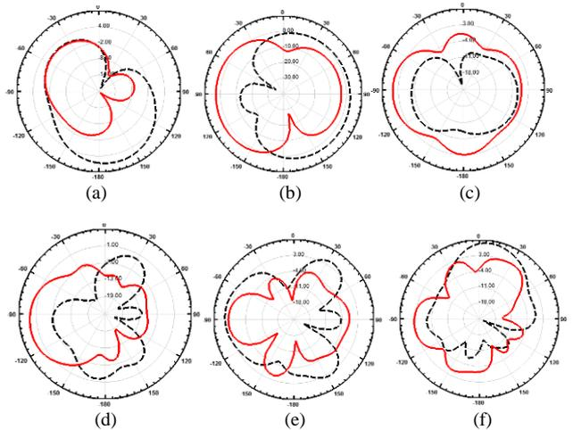
Fig 15: Simulated radiation patterns in H plane for antenna at different operating frequencies. (a) 4.1 GHz (b) 5.9 GHz (c) 9.5 GHz (d) 12.6 GHz (e) 13.5 GHz (f) 14.2 GHz
