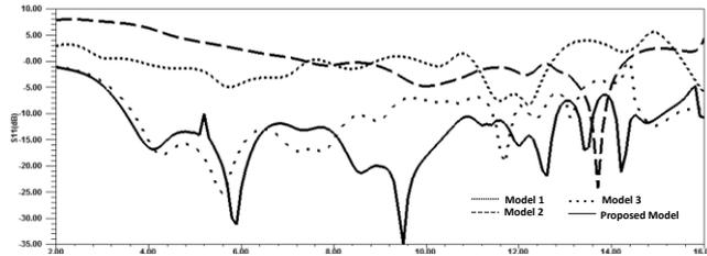
Fig 7: Return Loss Curve for all models.
