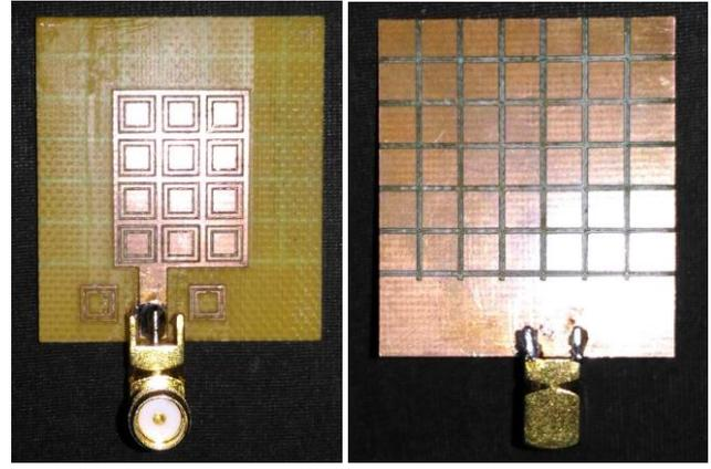
Fig 3: Prototyped Antenna (a): Fabricated Top Plane, (b): Fabricated Ground Plane
