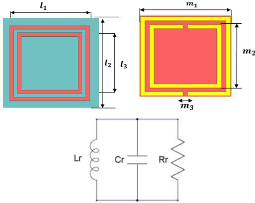
Fig 2 (a): Ring Resonators (b): CSRR (c):Equivalent Circuit
