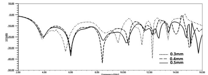
Fig 10: Simulated Return loss by varying slot width of ground
