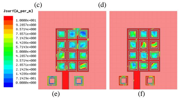
Fig 14: Simulated surface current distributions for antenna with different operating frequencies. (a) 4.1 GHz (b) 5.9 GHz (c) 9.5 GHz (d) 12.6 GHz (e) 13.5 GHz (f) 14.2 GHz
