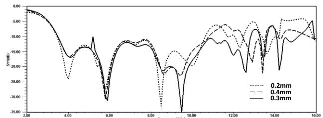
Fig 11: Simulated Return loss by varying width of splitters
