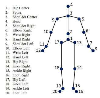
Fig 2. Skeleton template captured by Kinect sensor.
