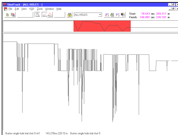
Fig.7: ShotTrack false VOD due to Reflection off joiner
