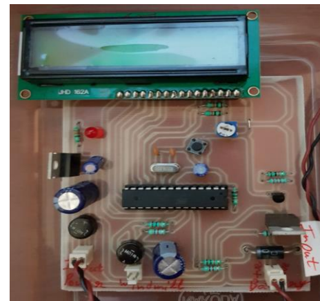
Fig. 5: Charge Controller Design Using ATMEGA 328.
