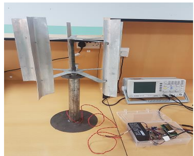
Fig. 6: Actual Laboratory Arrangement Involving the Proposed Design of VAWT.
