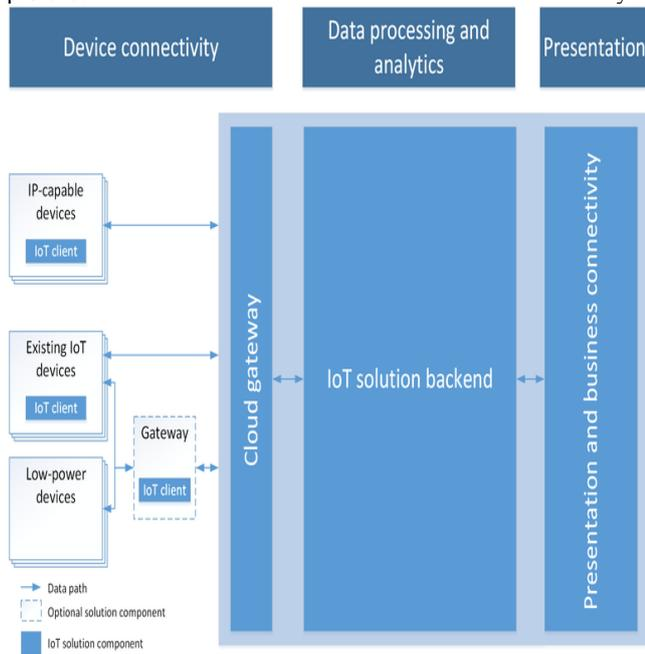
Figure 1.1: Architecture of IoT Hub
