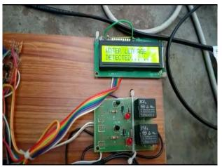
$\textbf{Fig.6} \ \text{Water leakage detected show in LCD}$
