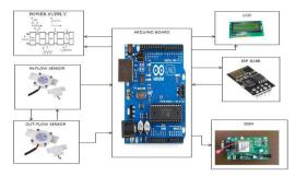
Fig.1 Block diagram of water system
