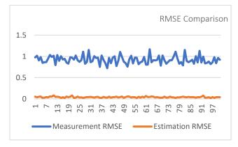
Fig. 7: Monte Carlo simulation for RMSE. Blue colored line indicates Measurement RMSE and the orange colored line indicates pendulum angle estimate.
