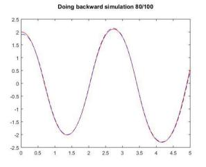
**Fig. 4:** Applying smoothing on filtered data for 80 times gives the smoothed better curve. The red line shows the true signal of pendulum and the blue dotted line indicates the dynamic trace that estimates the true signal.
