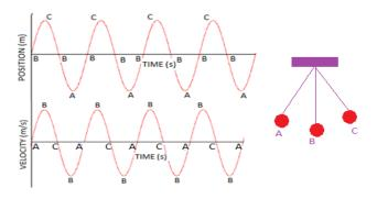
The accelerating positive peak is obtained when the bob is moving from B-C, and the decelerating positive position will be obtained when the bob moves from C-B (see position vs time plot above). Similarly, it follows negative peak in B-A and A-B path
