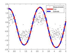
**Fig. 6:** Tracking signal simulation result. The red line indicates the target signal and the broken blue lines indicates the tracking signal. The time information is given by the horizontal axis and the pendulum angle is given by the vertical axis.
