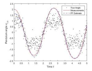
**Fig. 2:** Tracking based on particle filter estimation. The dots (.) indicates the true angle whereas the red line represents the measurement values and the blue lines states the estimated values of pendulum signal. Pendulum angle is taken along vertical axis and the horizontal axis is time axis in seconds.
