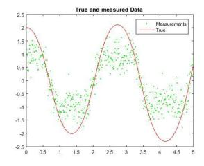
**Fig. 1:** Simulation result of pendulum wave equation with true and measured values. Red line represents true signal (to be tracked) and the green dots represents measured data points. The horizontal axis is considered as time axis and the vertical axis is referred as pendulum angle.
