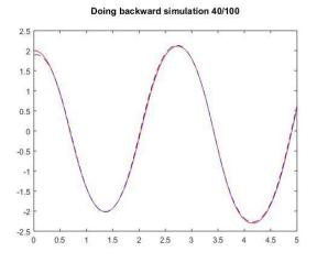
**Fig. 3:** Applying smoothing on filtered data for 40 times gives the smoothed better curve. The red line shows the true signal of pendulum and the blue dotted line indicates the dynamic trace that estimates the true signal.
