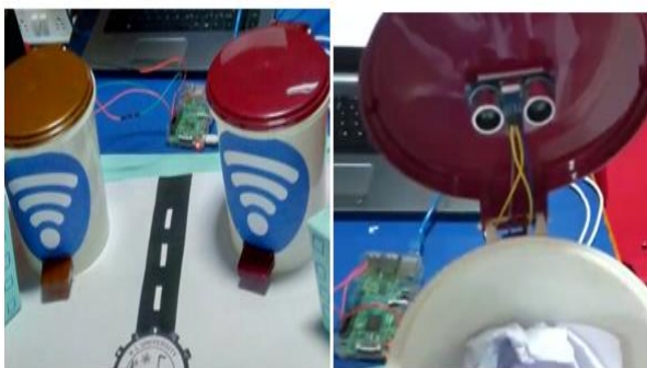
Fig. 2. dustbin with an ultrasonic sensor
