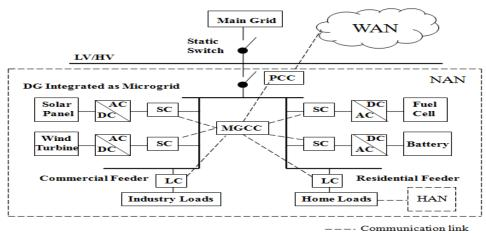
Fig. 1: Smart Microgrid Architecture.
