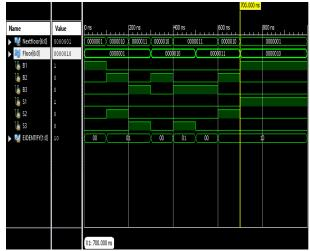
Fig. 10: Elevator Moving from Floor 3 to Floor 2.
