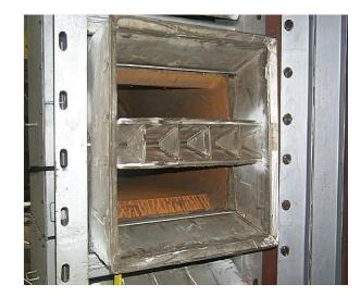
Fig. 2: Burner Nozzle
