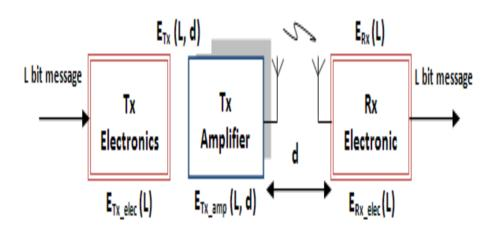
Fig.5: Radio Energy Dissipation Model
