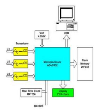
Fig. 2: Block diagram of the device
