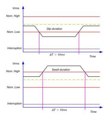
Fig. 1: The shapes of voltage dip and swell
