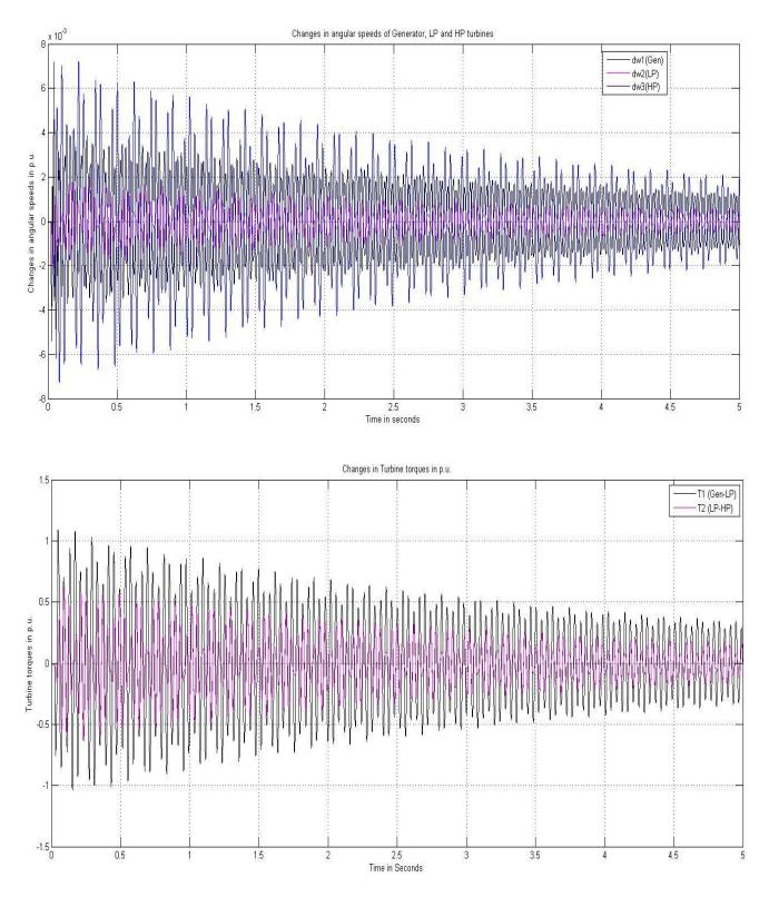
Fig. 4: Gen, LP, HP turbine outputs with respect to time with STATCOM
