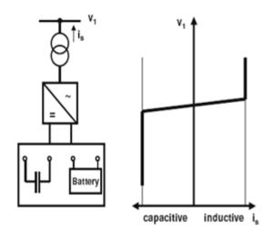
Fig. 1: Structure of STATCOM and voltage / current characteristic
