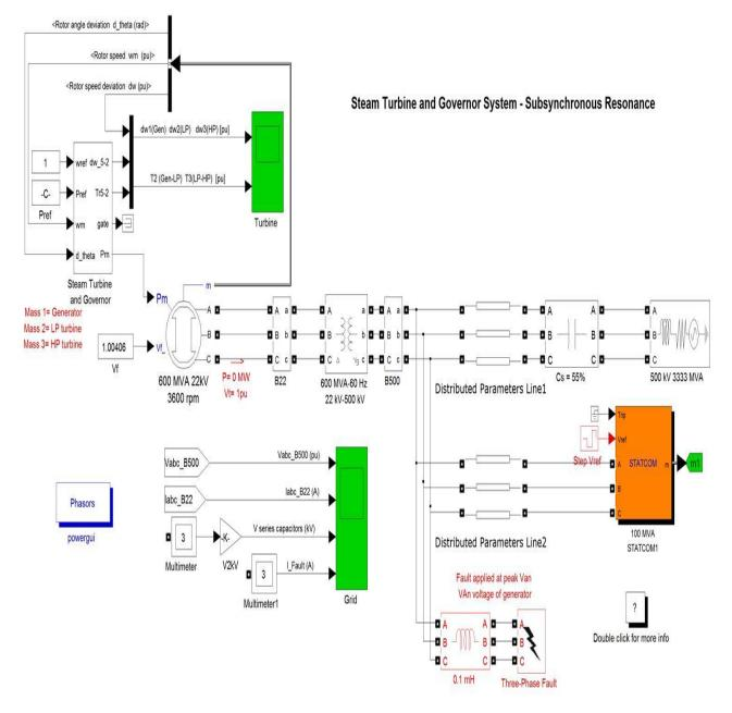
Fig. 3: Simulation circuit for the IEEE SBM system with STATCOM
