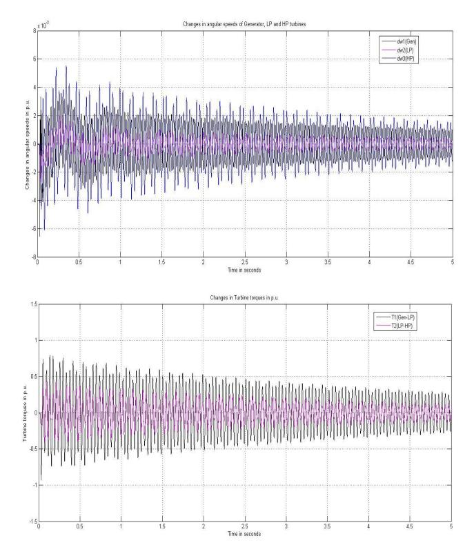
Fig. 9: Gen, LP, HP turbine outputs with respect to time with Unified Power Flow Controller
