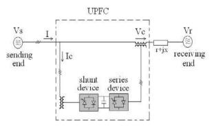
Fig. 7: Functional scheme of a basic UPFC
