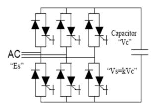
Fig. 2: STATCOM with Three Phase six pulse
