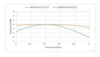
Fig 5. Insertion loss at port 2 and port 3
