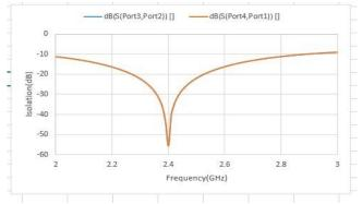
Fig 7. Isolation between ports 2 &3, ports 4& 1
