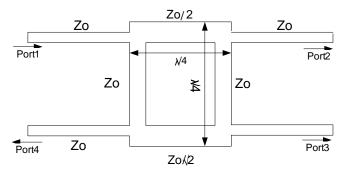
Fig1. Structure of quadrature hybrid coupler:  $Z_0$ = impedance of free space,  $\lambda$ =Operating Wave Length
