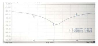
Fig 10. Isolation between ports 2 & 3, ports 4& 1
