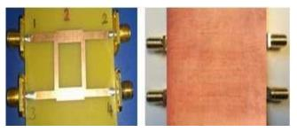
Fig 4. Fabricated patch hybrid front view and back view
