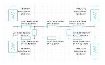
Fig 2. Schematic of proposed quadrature patch hybrid coupler: w=width of the Microstrip, p=length of the Microstrip
