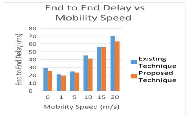
**Graph 5.3:** Comparison of End-to-End Delay Vs Mobility Speed.
