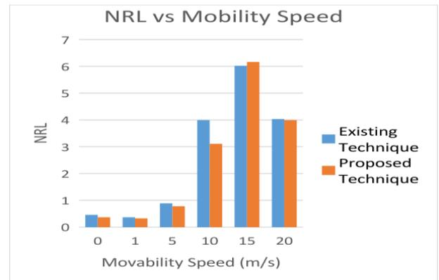
**Graph 5.2:** Comparison of the Normalization Load vs. Movability Speed.
