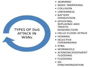
Fig. 2: Types of Denial of Attack in Wireless Sensor Network.
