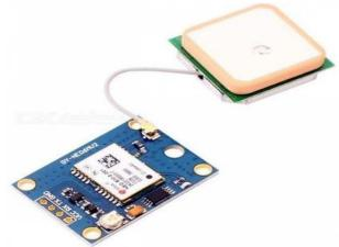
Fig. 3: Picture of GPS Module.
