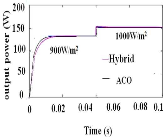
(b) ) PV power of proposed Hybrid MPPT with fast tracking
