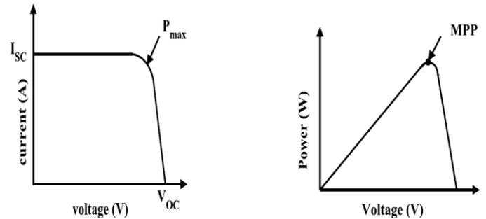
Figure 3 (a) I-V characteristics at  $1000\text{W}/\text{m}^2$  Figure 3 (b) P-V characteristics  $1000\text{W}/\text{m}^2$
