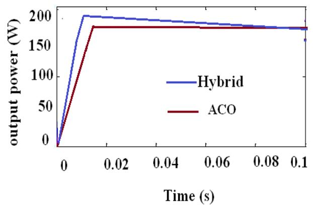
(b) ) PV power of proposed Hybrid MPPT with fast tracking
