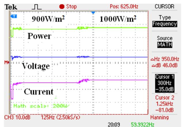
Fig. 14. Experiment results for 4S configuration for extreme rapidly changing insulation patterns of Hybrid-MPPT
