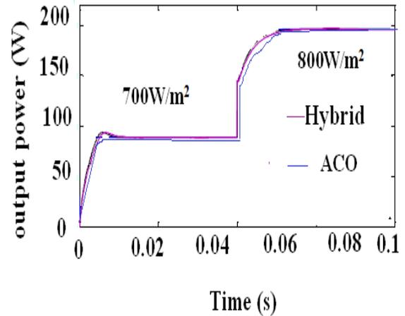
Fig. 10 Tracking curves for 4S series configuration (a) PV power of proposed Hybrid MPPT compared with other techniques
