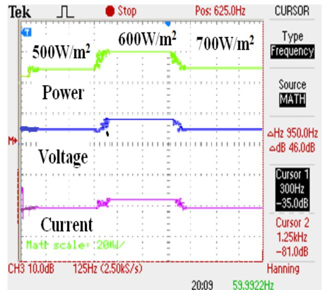
Fig. 12. Experiment results for 4S configuration for extreme rapidly changing insulation patterns of PO-MPPT
