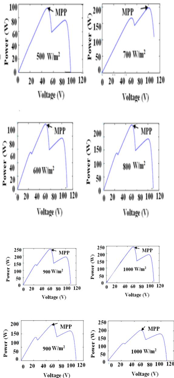
Fig. 5 P-V curves with MPP (a) 6S series configuration (b) 6S2P parallel configuration
