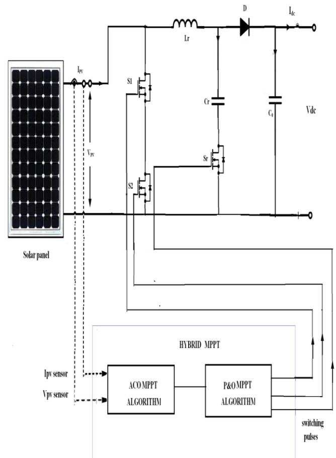
Fig. 8. Block diagram of proposed Hybrid-MPPT method
