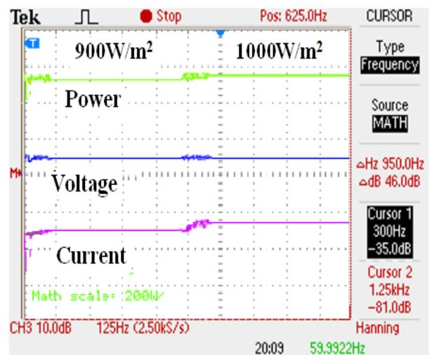
Fig. 13. Experiment results for 4S configuration for extreme rapidly changing insulation patterns of GWO-MPPT
