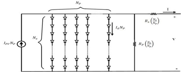
Figure 2: Series Parallel Combination of PV module
