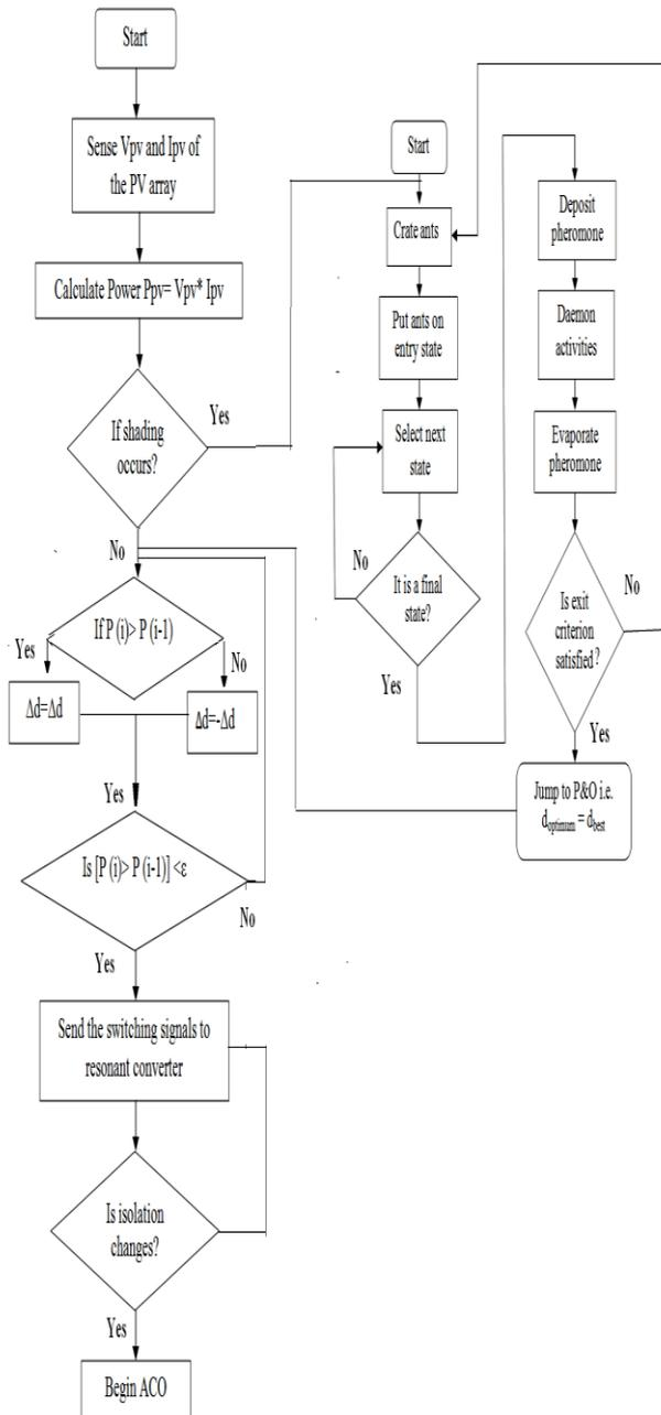
Fig. 7. Flowchart of the Hybrid-MPPT algorithm
