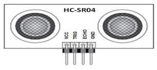
FIG. 3: Ultrasonic Sensor HC-SR04.
