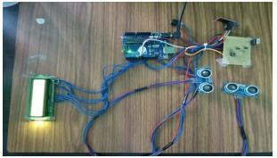
Fig. 7: Arduino Board Interfacing with LCD.
