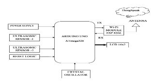
Fig. 1: Architecture of Smart Dust Bin.
