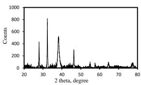
**Fig. 5:** XRD Diffraction of AgNPs Powder Synthesized at the Suitable Conditions and Dried at 60 °C.
