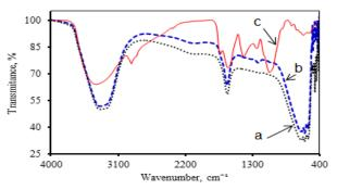
Fig. 4: FT-IR Spectra of F.J. Extract (A), AgNPs Solution (B) and AgNPs Powders (C) Synthesized at the Suitable Conditions.
