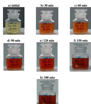
Fig. 2: By-Time Colour of AgNPs Solution (V = 50 mL; 3.0Ag/2.0Ext; T = 35 °C; Sunlight; V<sub>stir</sub> = 300 Rpm; C<sub>ag+</sub> = 1.0 mM).
