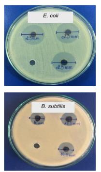
Fig. 7: The Diameter of the Zone Observed Against E. Coli. and B. Subtilis of AgNPs Sample Synthesized at the Suitable Conditions.
