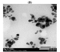
Fig. 6: SEM (A) and TEM (B) Images of AgNPs Synthesized at the Suitable Conditions.
