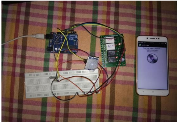
Fig. 9: All OFF Condition using Bluetooth and PIR.
