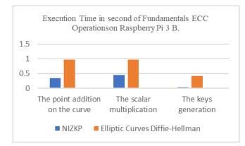
Fig. 3: Execution Time in second of Fundamentals Elliptic Curve Operations on Raspberry Pi 3 B.
