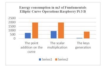
Fig. 4: Energy consumption in mJ of Fundamentals Elliptic Curve Operations Raspberry Pi 3 B.
