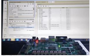
Fig. 17: Implementation of proposed method using VIO Core Logic analyzer
