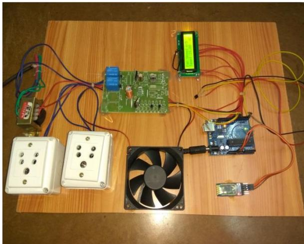
Fig. 8: Experimental Setup for Fan (Off Mode) with Normal Temperature.
