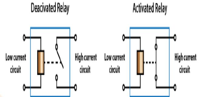
Fig. 4: Relay Circuit Diagram.
