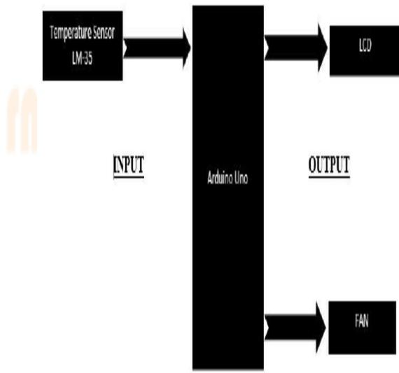
Fig. 1: Block Diagram of Fan Speed Control System.
