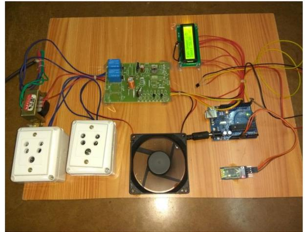
Fig. 9: Experimental Setup for Fan (On Mode) with Excess Temperature.
