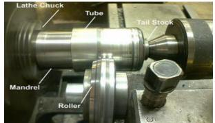
Fig. 1: Single Roller Flow Forming Lathe Machine [9].
