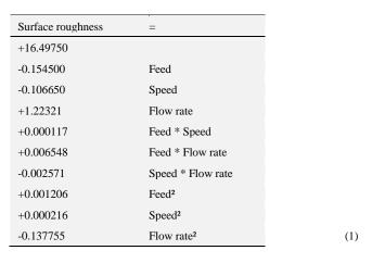
The equation 1 shows the quadratic mathematical model of surface roughness in terms of feed, speed and flow rate of coolant.
