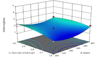
Fig. 4: Response Graph of Flow Rate of Lubricant and Speed at Feed 60  $\rm Mm/Min.$
