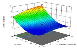
Fig. 3: Response Graph of Feed and Flow Rate of Lubricant at Speed 250 Rpm.
