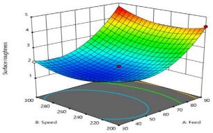
Fig. 2: Response Graph of Speed and Feed at Coolant Flow Rate of 3.08 L/Min.
