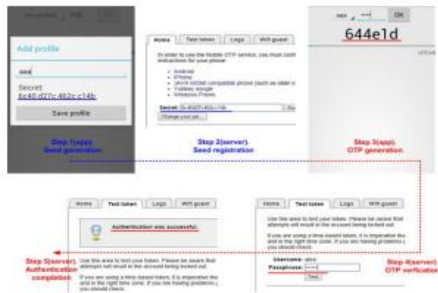
Fig. 4: Verification procedure of OTP generation
