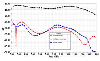
Fig. 3: S<sub>21</sub> parameter of proposed antenna
