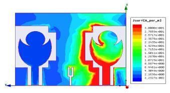
Fig. 6 (a): Current distribution at 3.1 GHz.
