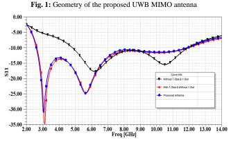
Fig. 2:S<sub>11</sub> parameter of proposed antenna
