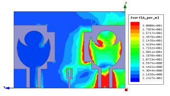
**Fig. 6** (c): Current distribution at 10.6 GHz. **Fig. 6**: Current distribution when port 1 excited.
