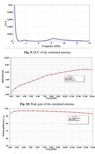
Fig. 11: Radiation efficiency of the simulated antenna.
