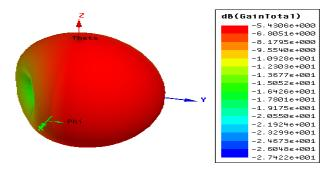
Fig. 7 (a): 3-D polar plot at 3.1 GHz.
