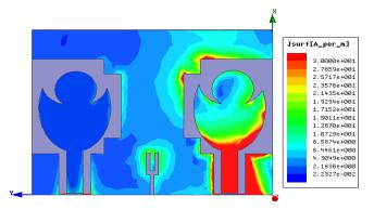
Fig. 6 (b): Current distribution at 5.6 GHz.
