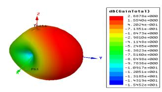
Fig. 7 (c): 3-D polar plot at 10.6 GHz.
