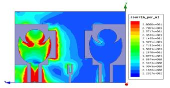
Fig. 4 (c): Proposed antenna.
