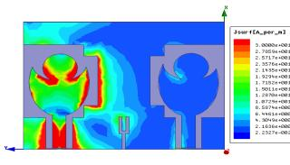
Fig. 5(c): Current distribution at 10.6 GHz.Fig. 5: Current distributions when the port 1 is excited.
