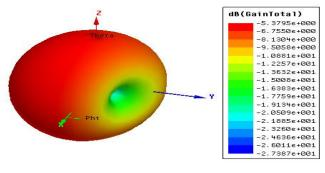
Fig. 8 (a): 3-D polar plot at 3.1 GHz.
