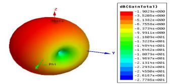
Fig. 8 (b): 3-D polar plot at 5.6 GHz.
