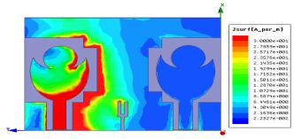
Fig. 5 (a): Current distribution at 3.1 GHz.
