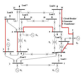
Fig. 3: IEEE 14 Bus Reliability Test System.
