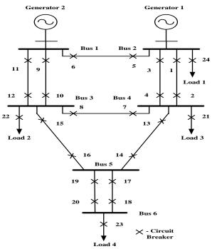
Fig. 2: IEEE 6 Bus Reliability Test System.
