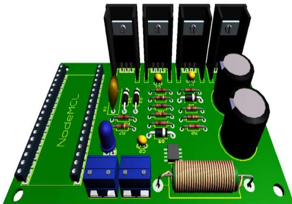
**Fig. 11:** Three-Dimensional Module of the Client Controller.
