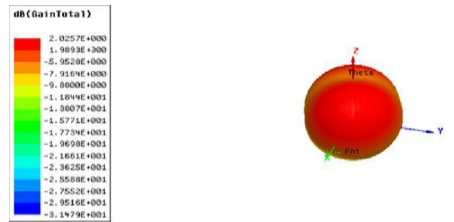
Fig. 22: Gain for the coaxial feeding
