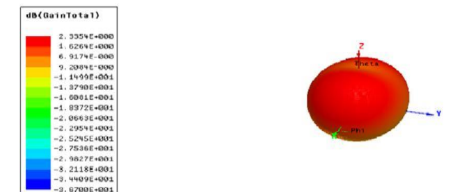
Fig. 24: Gain for the coaxial feeding with DGS and DSS
