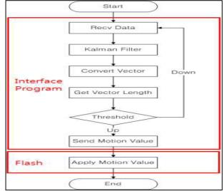
Fig. 10: Flowchart of Motion Recognition.
