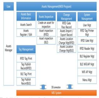
Fig. 9: Web Program Menu Configuration of Smart Asset Management System.
