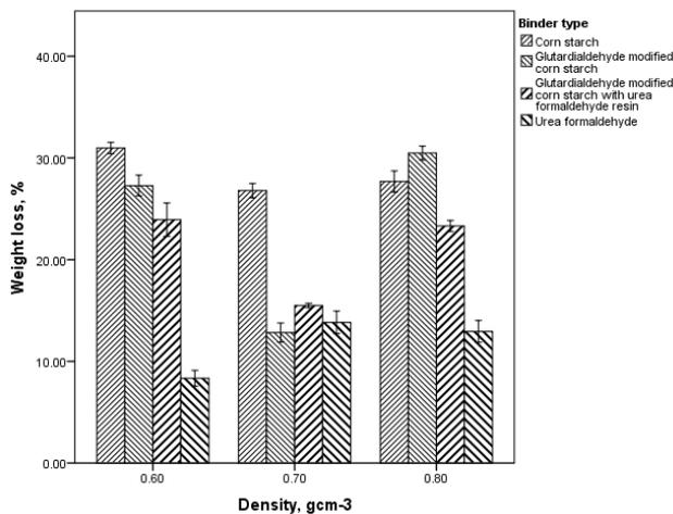
Figure 4 Weight loss of particleboard after exposure to *Trametes versicolor* fungal.
