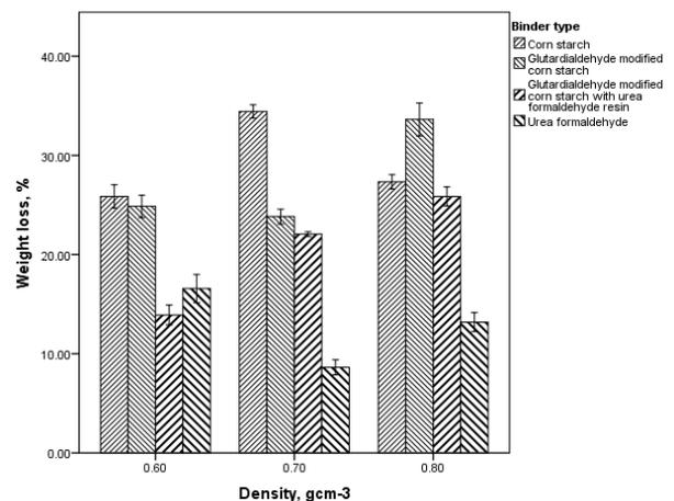
Figure 2 Weight loss of particleboard after exposure to *Pycnoporus sanguineus* fungal.
