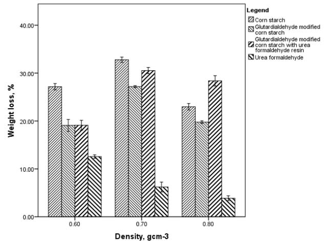
Figure 1 Weight loss of particleboard after exposure to *Formitopsis palustris* fungal.
