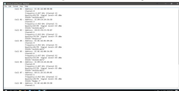
Fig. 7: Result from scanning the available access point
