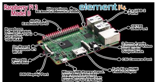
Fig. 3: Raspberry Pi Model B
