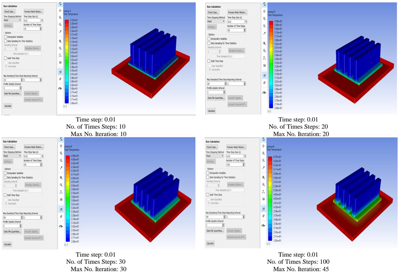
Fig. 4: Graph plot of temperature distribution of heat sink at number of times step and max number of iteration.
