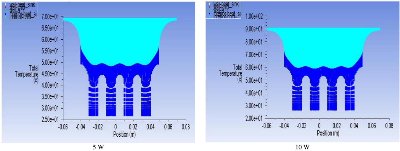
Fig. 3: Graph plot of temperature distribution of heat sink at different chip power.
