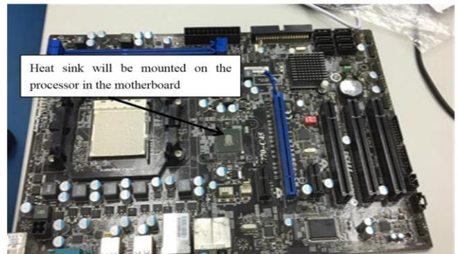
Fig. 1: Simulation setup for heat sink mounted on the motherboard (top view).
