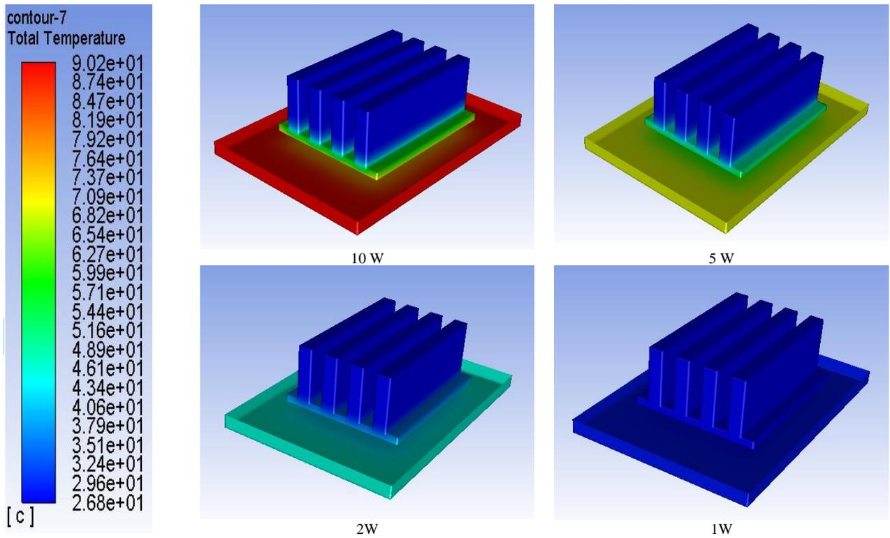
**Fig. 2:** Temperature distribution of heat sink using chip power 1 W to 10 W.
