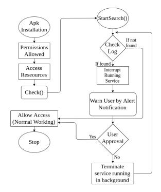
Fig. 2: Background Process Monitoring through Android Log
