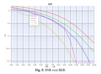
The achievement of SNR over BER is shown in Fig.5. The BER response of FBMC was much better than OFDM and UFMC. At 1e-4 of BER, the SNR of FBMC was decreased by an amount of 1.6 dB to UFMC, 3dB to F-OFDM and 5.5 dB to OFDM. It was realised that the FBMC BER response has been nearer to the theoretical response such as QPSK BER.
