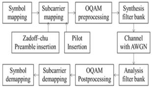
Fig. 1: Proposed Block Diagram for FBMC.
