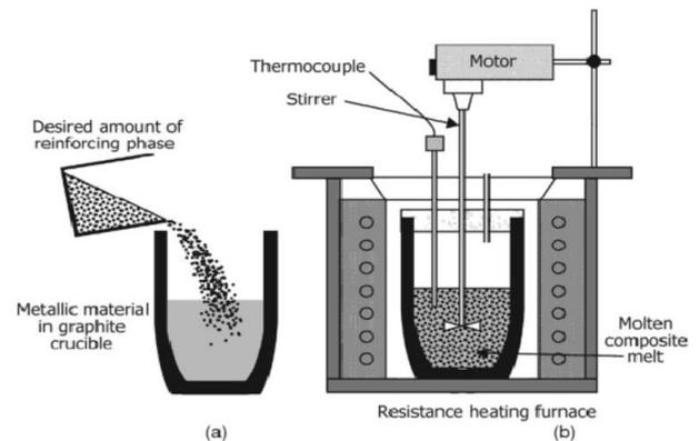
**Fig. 1:** (A) Mixing of CNT Powder in Molten Aluminium Metal. (B) Resistance Heating Furnace with Motorized Stirrer for Uniform Mixing of Reinforced CNT in Al Matrix.
