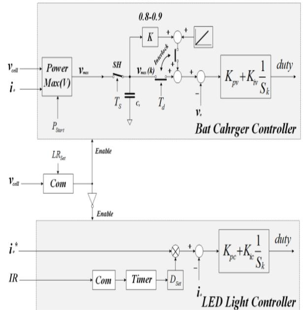
Fig. 6: Solar Street Light System Control Block Diagram.
