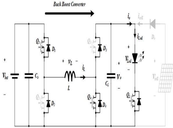
Fig. 4: DC / DC Converter System Circuit according To Operation Mode.
