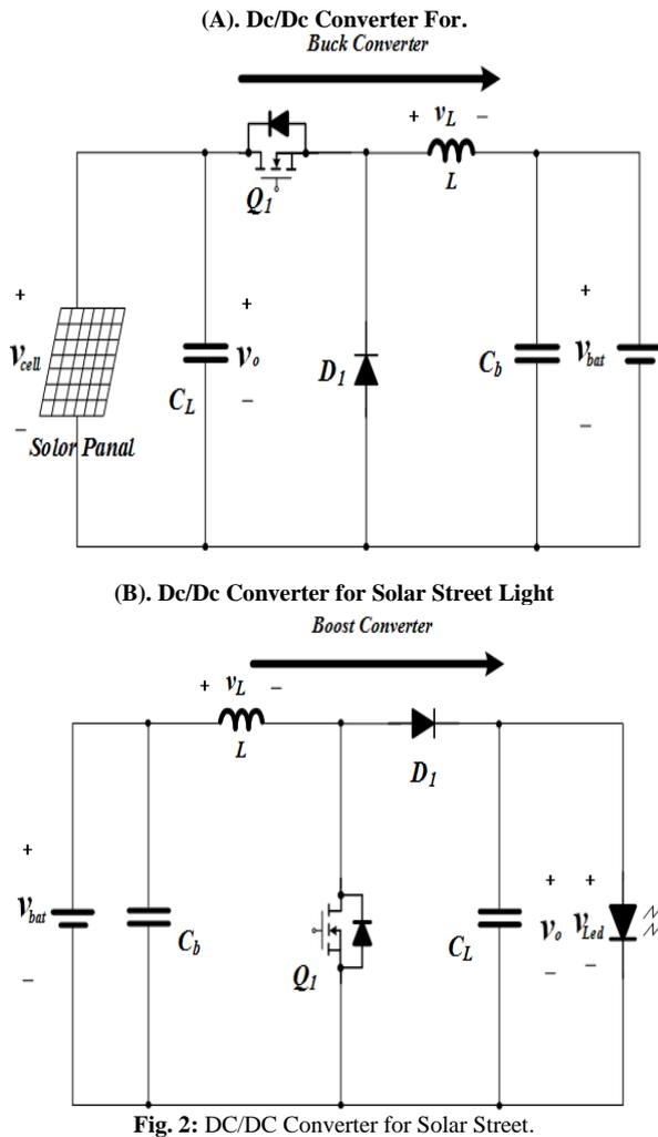
Fig. 2: DC/DC Converter for Solar Street.
