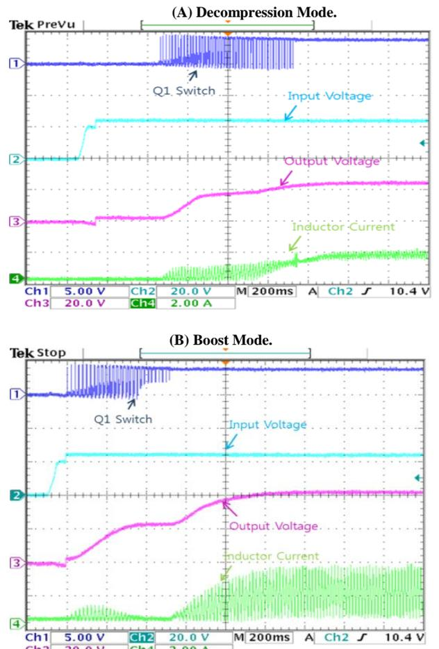
Fig. 8: Converter Starting Characteristics for Solar Streetlight.
