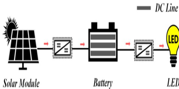
Fig. 1: Schematic of a Typical Stand-Alone Solar Streetlight.
