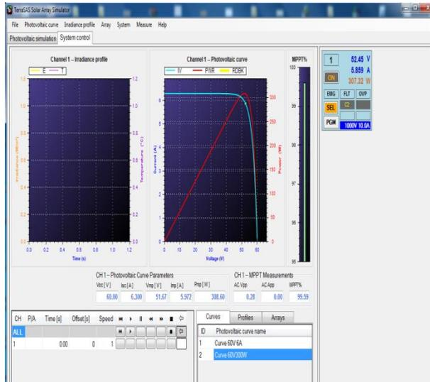
Fig. 10: MPPT Tracking Characteristics.
