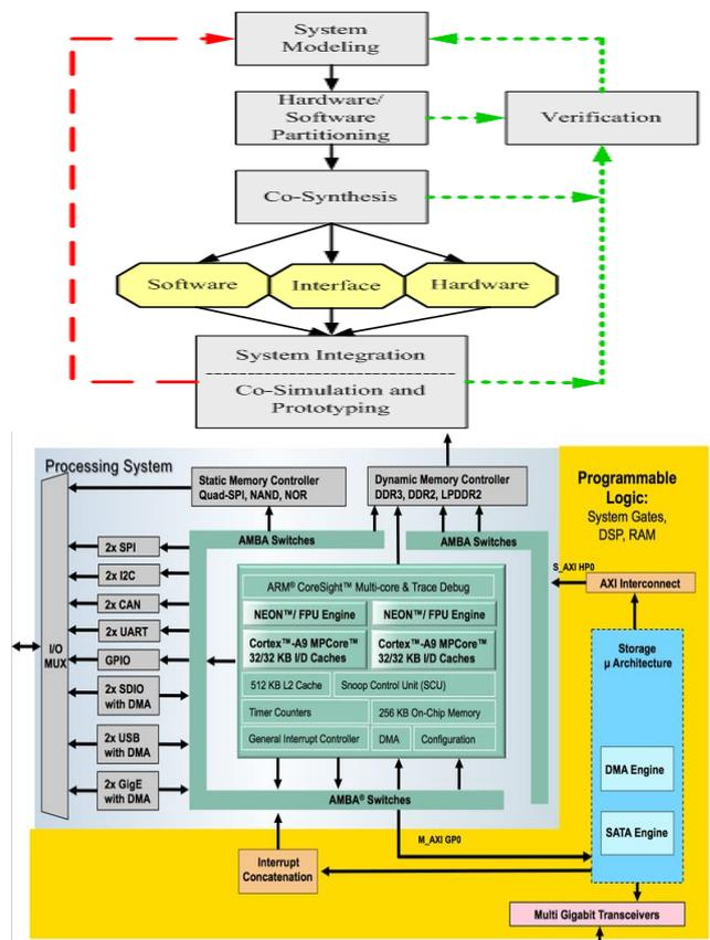
Figure 3: Hardware/software co-design flow
