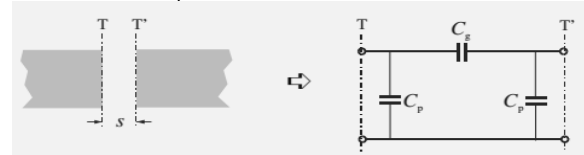
Figure.3 Microstrip gap discontinuities.
