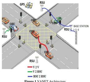
The second structure is 'vehicle to RSU' where either of transceiver is vehicle and infrastructure wireless component like RSU. In which RSU is used to collect information from vehicles and provide that information to other vehicles when necessary. The Hybrid structure is that a vehicle or RSU communicates with other nodes in single hop or multi hop.
