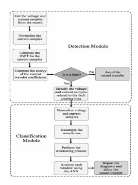
Fig1. Fault detection and Classification in Transmission line
