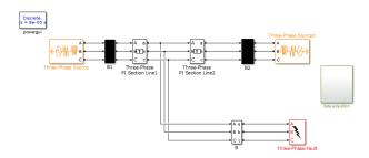
Fig (1):consider transmission line which is length 300Km which has two sources on bothside with voltage 400volts.
