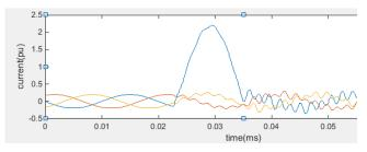
**Fig(3):** when there is flaw in phase A we observe that the current in phase A is more when compared to other phases.
