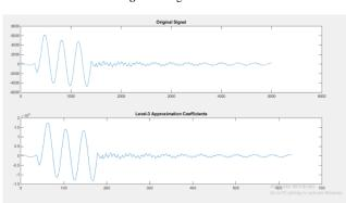
Fig 9: Current at Phase- A after using Wavelet change(LG-Fault)
