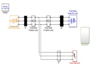
Fig 3: MATLAB Simulation Block diagram
